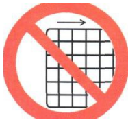
Figure 6 - Warning label - do not operate with guard removed
