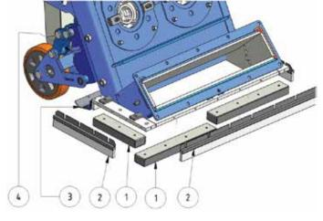
over the floor surface depending on the application. This is also very important for the best function of the machine. The adjustment is done by set screws on the traction drive and the rear (4).
