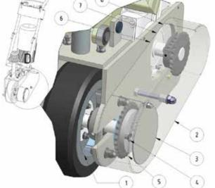
quick release pin (4) will link these parts so the energy gets to the drive wheel.
