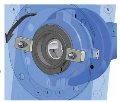
The Control Cages, held by two clamps (4) need to be adjusted so the blast pattern shows to the center of the machine and gives an optimal blasting result.
