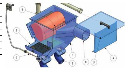
The Separator (1) is mounted to the end of the Rebound plenum. The deflector (5) and Baffle Plate (4) stop the reflected abrasive.
