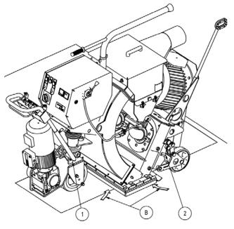
The height of the brush seals should be maximum 1 mm above the surface. The adjustment is possible within the slots of the seal elements. The setting depends on the structure of the surface to be treated, in general the rougher the surface the lower the setting. Working on steel means to set it down as far as possible.
