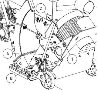
(See Figure on following page): Please use only appropriate, allowed, and qualified hoisting equipment (A) as well as ropes and chains (A). See Chapter 1 for the weight of the equipment or look on the serial plate of the machine. Do not fix any rope or chain (A) to the handle. Fix ropes and chains only at locations as shown in the next figure.
