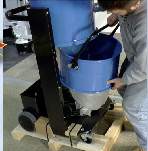
Uses Longopac bags to catch fine dust particles for easy disposal
