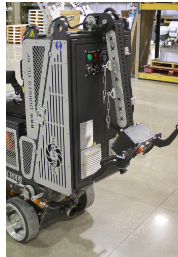
Lower Position: for remote operation and transportation
