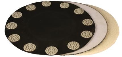
The CASH Dot Pad is a rubber disc with individual resin pads fixed to it and has hook Velcro on the reverse side. The CASH Dot pads are only to be used with water and NEVER dry. This tool is used to perform concrete polishing, marble polishing and terrazzo polishing that is smooth, cured and free of any sealer or coating and moderately worn marble or terrazzo floors. The CASH Dot System is engineered to be run on a high speed, propane or electric, burnisher, swing machine, or auto-scrubber.
