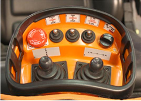
The remote control is very simple to operate. Without interrupting the grinding, the operator can handle smaller tasks of a phone call or adjusting the dust collector while keeping to the overall project. This doubles his capacity to handle the job effectively and efficiently.
